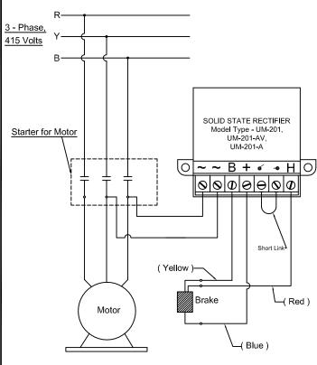
Connection Schematic (with purely A C Switching)
