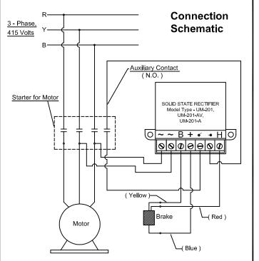
Above schematics are with AC cum DC switching for fast disengagement and fast engagement of the brake.
